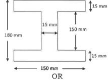
Q.5(B) Determine the centroids and moment of inertia of the area shown in 10M 4 4 Figure with respect to its centroidal axes.
