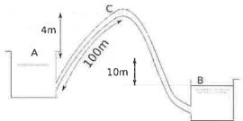
Q.4(B) Find the rate of flow through the siphon pipe and also find pressure at point C. Diameter of the pipe is 20cm. Total length of pipe is 600m. Take f=0.006. Neglect minor losses.
